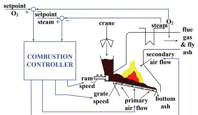
Fig. 2: A typical MSWC plant combustion controller
