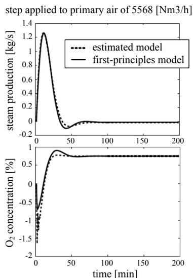
Fig. 5: Responses of steam and  $O_2$  to step on primary air flow
