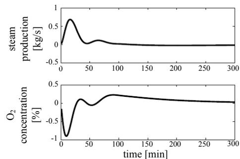
Fig. 8: An example result of loop shaping: 'mirrored' CV responses to same step applied to pre-filtered air flow inputs
