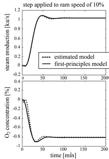
Fig. 3: Responses of steam and O<sub>2</sub> to step on ram speed
