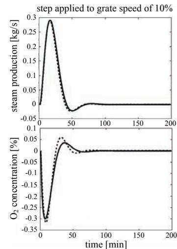
Fig. 4: Responses of steam and O<sub>2</sub> to step on grate speed
