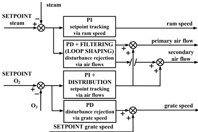
Fig. 7: The new PID combustion control strategy
