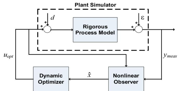
Fig. 1. Output feedback model-based control framework.
