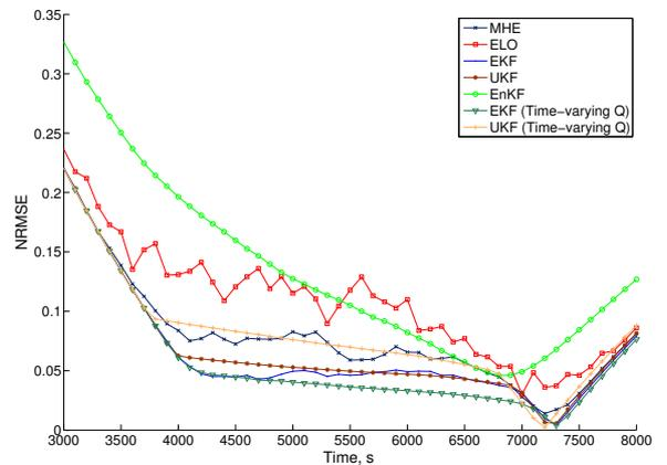
Fig. 4. Errors in the reference crystal growth rate trajectory tracking under the uncertain scenario.
