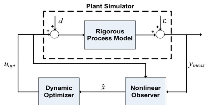
Fig. 1. Output feedback model-based control framework.
