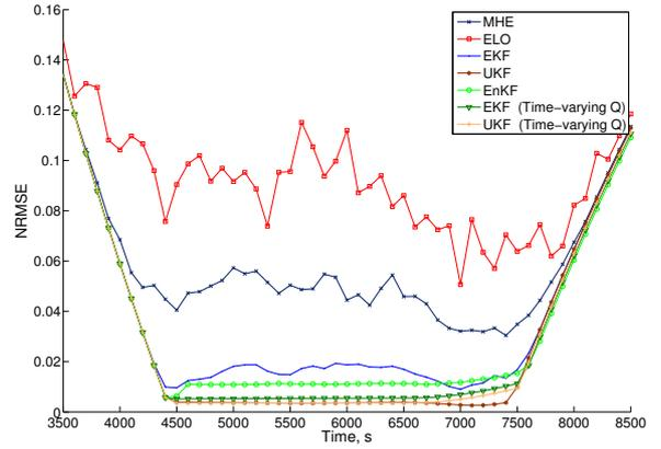
Fig. 3. Errors in the reference crystal growth rate trajectory tracking under the nominal scenario.
