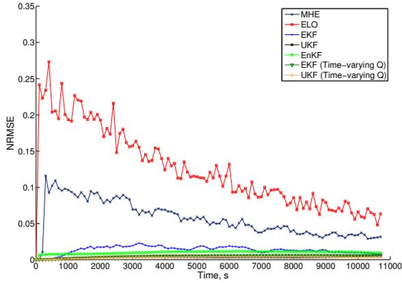
Fig. 2. Estimation errors of the 2<sup>nd</sup> moment of CSD under the nominal scenario.
