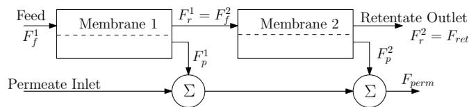
Fig. 1. The two membrane stacks system.
