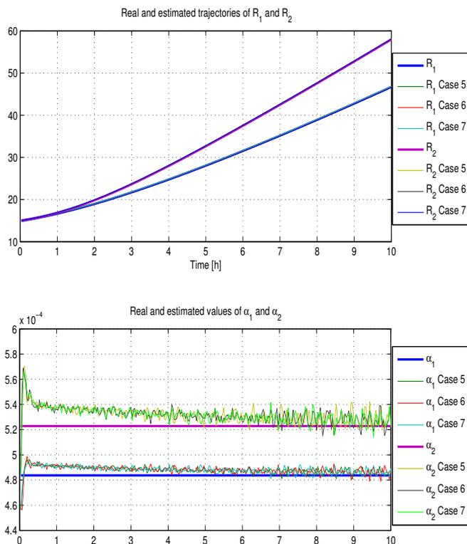
Fig. 4. Simulation results for membrane system. The upper figure visualizes the true and estimated membrane resistance (state) trajectories while bottom figure visualizes the true and estimated fouling coefficient (parameter) trajectories for output channel cases 5, 6 and 7.
