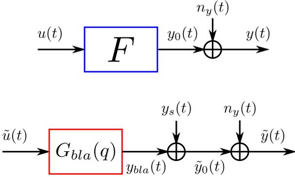
Fig. 2. A dynamic nonlinear system ( $F$ ) with zero-mean (colored) additive noise  $n_y(t)$  at the output only (top) is represented as the Best Linear Approximation of the system behavior  $G_{bla}(q)$  and a stochastic nonlinear distortion source  $y_s(t)$  (bottom).
