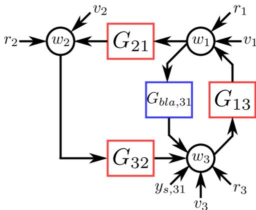
Fig. 7. The BLA representation of the example nonlinear dynamic network with 3 nodes (see Figure 1). The nonlinear subsystem  $F_{31}$  is replaced by its BLA and a stochastic nonlinear distortion source  $y_{s,31}$  is added to node 3.
