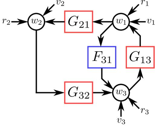
Fig. 1. An example of a nonlinear dynamic network with 3 nodes. The node signal  $w_i(t)$  is obtained as the sum of the outputs  $y_{ij}$  of the linear  $G_{ij}$  and nonlinear  $F_{ij}$  subsystems connecting to it, the noise signal  $v_i(t)$  and the known reference signal  $r_i(t)$ .
