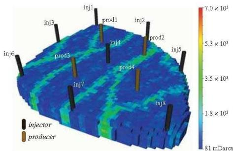
**Figure 1: Permeability field of realization 1 of a set of 100 realizations ([12],[27]). The permeability is expressed in mDarcy =  $9.87 \times 10^{-16} m^2$ .**
