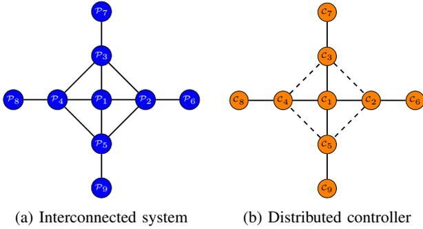
Fig. 3: Graph for the interconnected system (a) and distributed controller (b) that satisfies Assumption III.1 (solid and dashed edges), with a reduced number of communication links (solid edges) and a decentralized controller (no edges).
