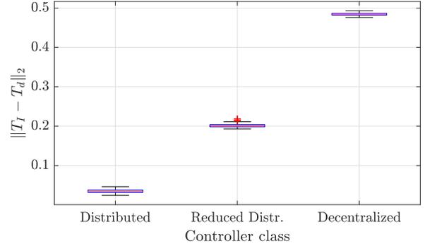
Fig. 5: Distribution of the achieved performance for various controller classes, where  $T_I$  and  $T_d$  denote the transfers  $r \rightarrow y$  and  $r \rightarrow y_d$ , respectively. From left to right: a distributed controller satisfying Assumption III.1, a controller with four communication links removed and a decentralized controller.
