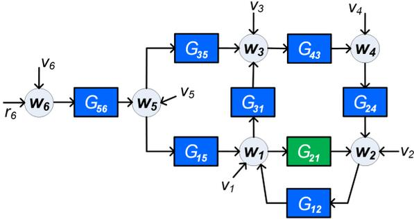
Fig. 1. Example network with the green module  $G_{21}$  being the target module for identification (Ramaswamy and Van den Hof (2019)).
