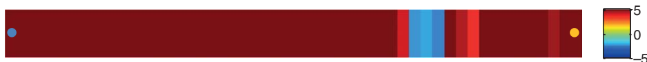
Fig. 4—Updated permeability field of the 1D reservoir model for Experiment No. 2. Permeability values are expressed as the natural logarithm of permeability in md.
