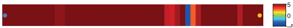
Fig. 5—Updated permeability field of the 1D reservoir model for Experiment No. 3. Permeability values are expressed as the natural logarithm of permeability in md.
