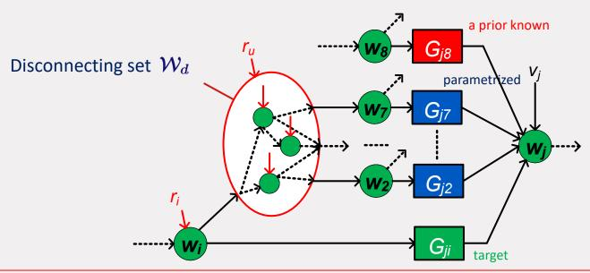
**Result**<sup>[1]</sup>:  $G_{ji}$  is generically identifiable if independent external signals are added to the nodes in  $\mathcal{W}_d$  and  $w_i$ . This can be either (independent) noise signals designed excitation signals.
