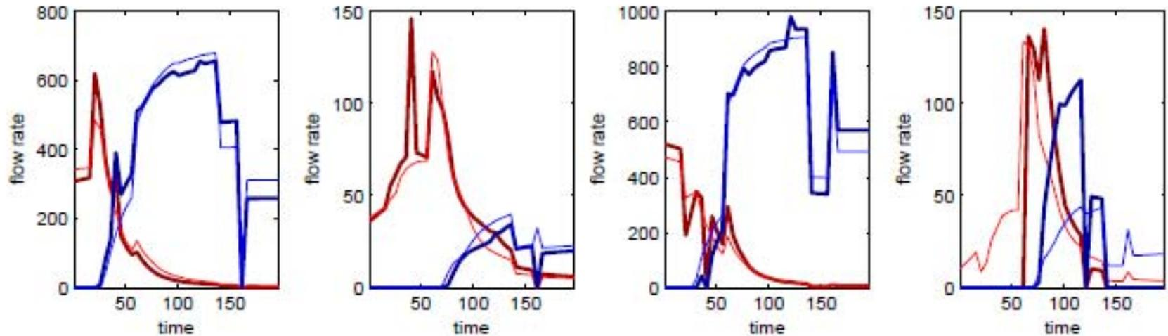
Simulated production of estimated model (thin lines) of water (blue) and oil (red) in the four producer wells
