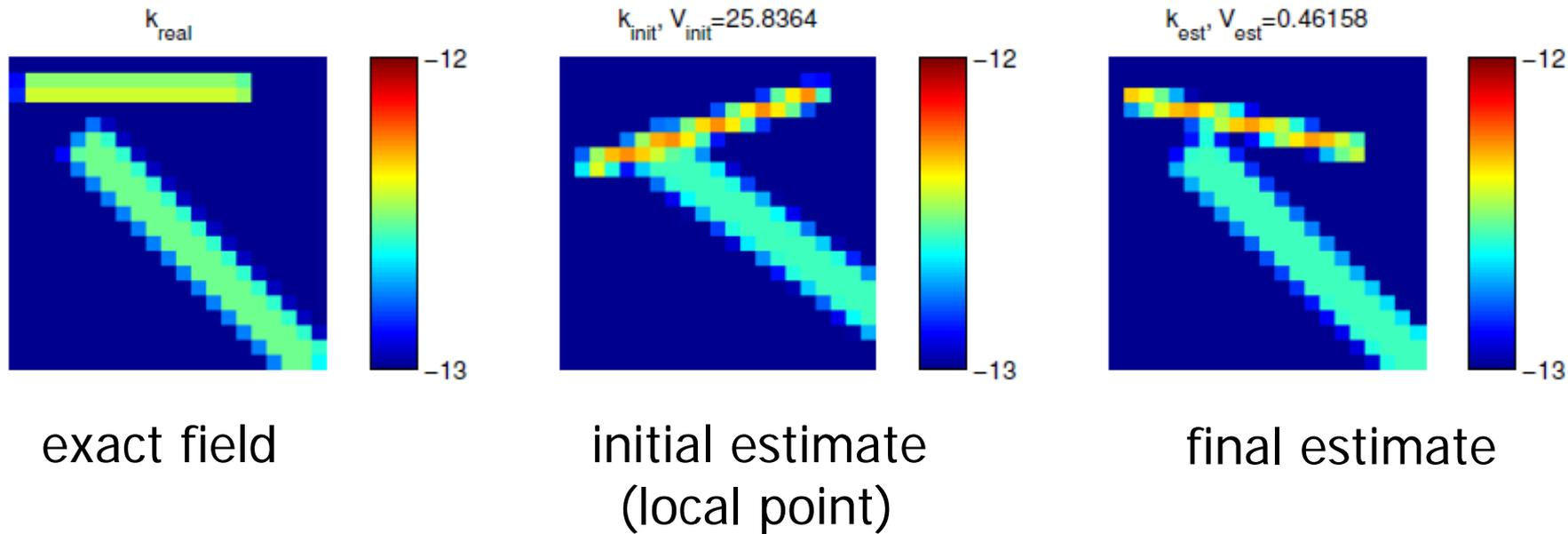
Parametrization of two straight channels with variable position and orientation, and single permeability value (total 13 param)
